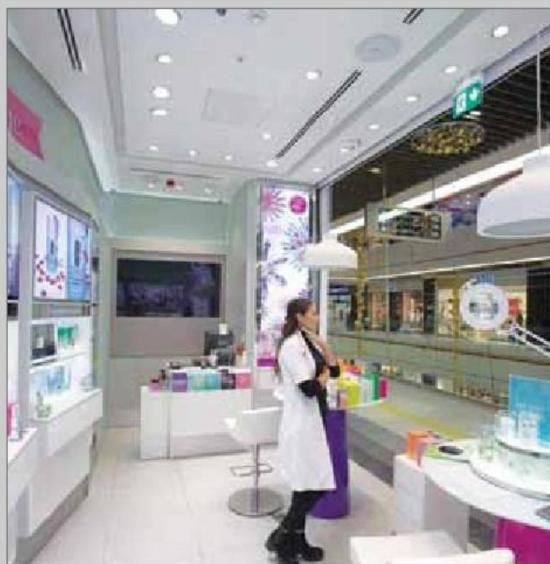
Especially with the use of square shaped embedded luminaires, it was possible to deliver an architectural style compatible with the ceiling structure of the Bobbi Brown store. Luminaires with 12W LED bulbs were adjusted with 18o in order to lay emphasis on the mid-level displays while they were adjusted to 30o reflector angle for the remaining areas.
