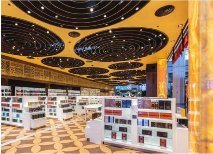
ensured by correct power and reflector angles while all illumination devices were placed on the current beams. In these spaces, 25W and 30W PrideLed rail spots with luminous color of 3000 Kelvin were used.
